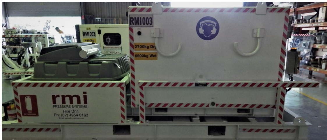
2. Diesel Tank Skid
